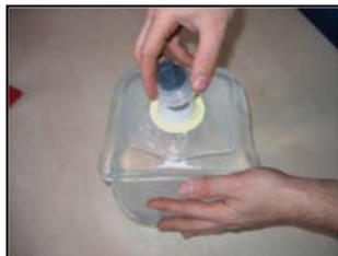
Fig. 15: Screw on the Canister connection for brine coupling
