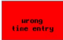
Fig. 45: Wrong time entry time switch
