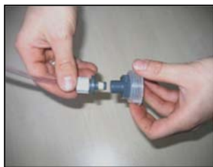
Fig. 14: Pull off the Canister connection for brine coupling
