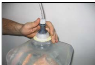
Fig. 16: Insert the suction line
